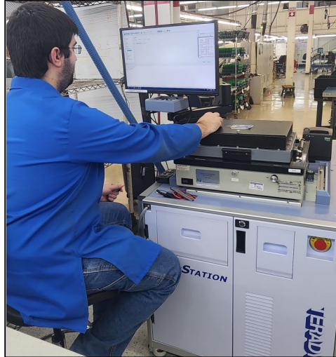
The new ICT has a small footprint and is compatible with legacy product test fixtures and programming.
