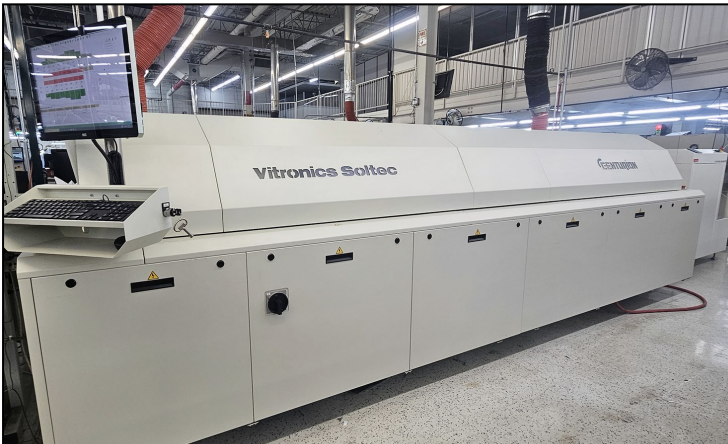
EGV now has two forced convection reflow ovens that can do both nitrogen and air soldering.
